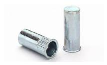
Highest resistance to vibration and spin out of all round bodied rivnuts. Flange are wide and near flush finish. Very wide grip range.
